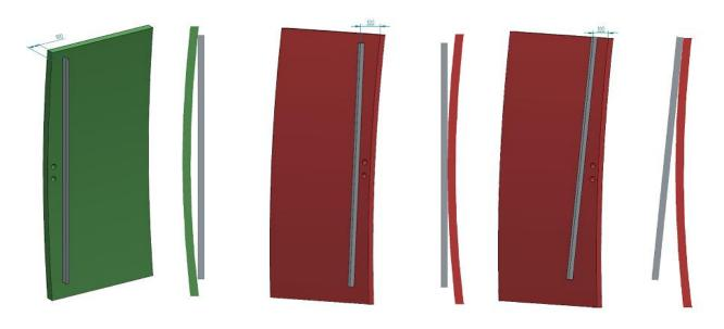
The permitted curvature of the door panel is 2 mm per meter.
